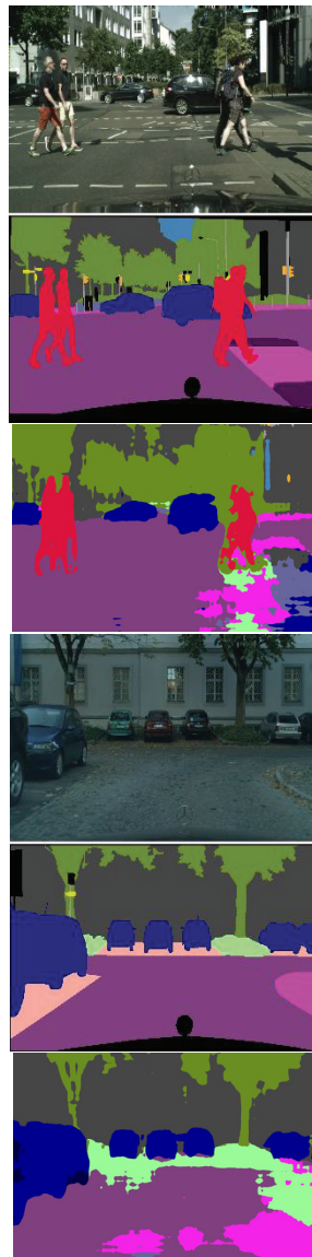
Fig. 5. Domain adaptation semantic segmentation performed on Cityscapes dataset. The first row represents the raw images. The second row represents the ground-truth semantic segmentation (provided by Cityscapes dataset). The third row represents semantic segmentation achieved by our model.
